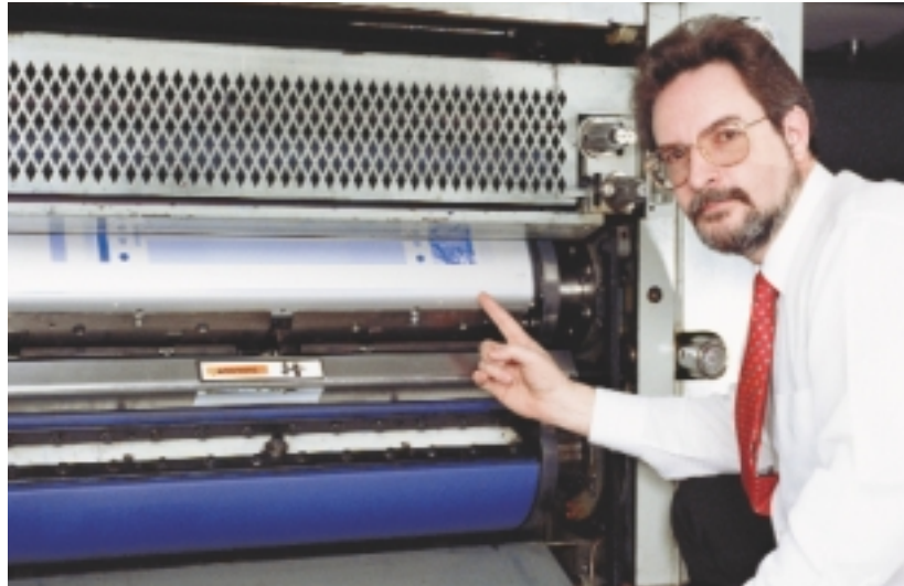
A thin scum line on the plate bend indicates good ink/water balance.
